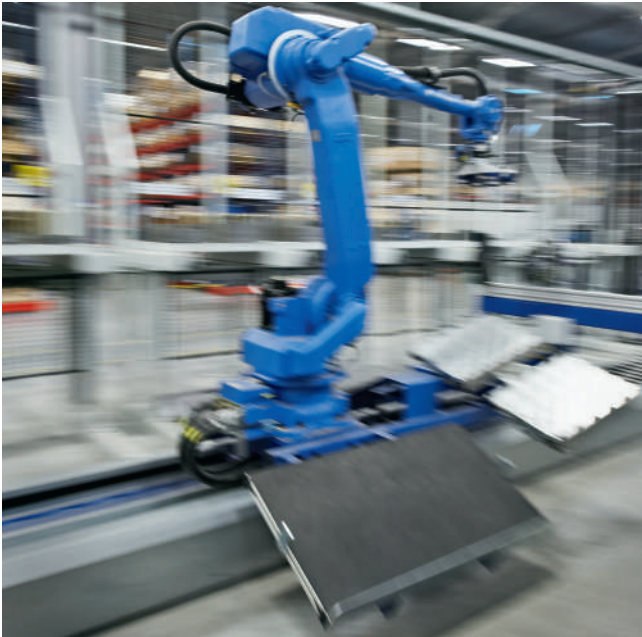
Press brake application with a robot and accompanying equipment that travels on the servo powered track.
