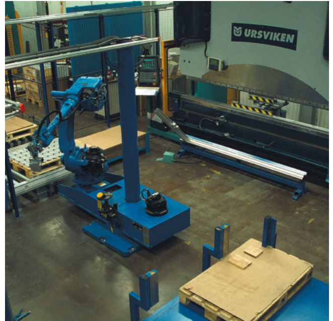
Increased working range for the robot mounted on a VST rotating base.
